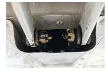
provide lightning protection by allowing current to pass through the airframe with minimum arcing.
